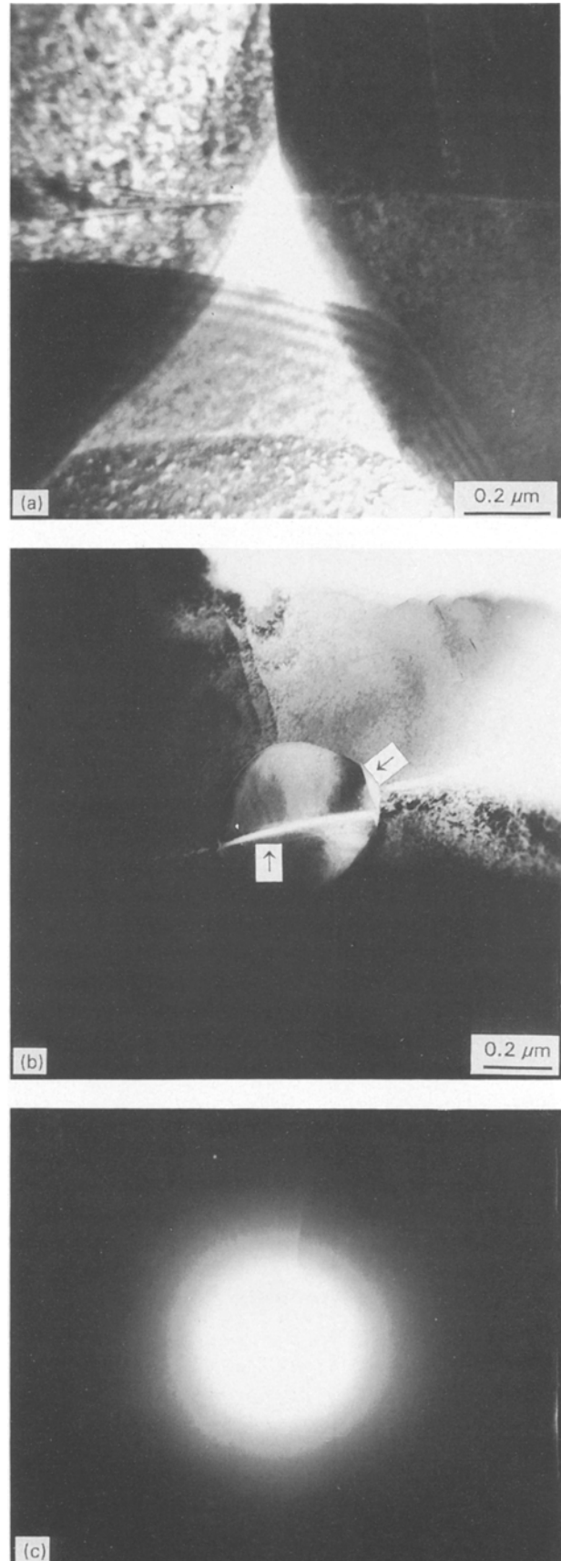
Figure 4 Transmission electron micrographs of amorphous grain-boundary phases. (a, b) Bright-field image, (c) SADP. The arrows indicate the grain-boundary phases.
